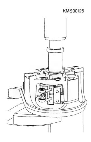
CHECKING AND REPAIRING COMPONENTS Checking commutator end shield Installation: Use reversed pressingout and pressing-in mandrel to press in new bushing. ATTENTION: Bushing must have been impregnated beforehand for 8 hours with Shell Tellus oil. Pressing-out and pressing-in mandrel for bushing in commutator end
